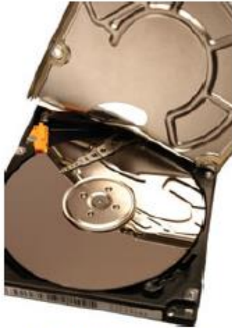
Hard drive with enclosure opened
