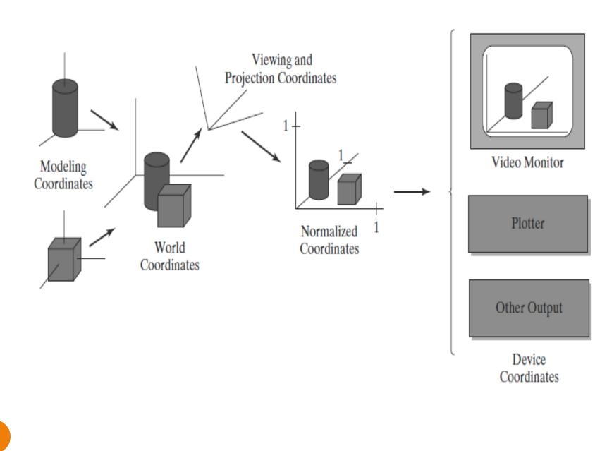
This step involves the transformation of the individual modeling-coordinate frames to specified positions and orientations within the worldcoordinate frame. Geometric descriptions in modeling coordinates and world coordinates can be given in any convenient floating-point or integer values, without regard for the constraints of a particular output device.
