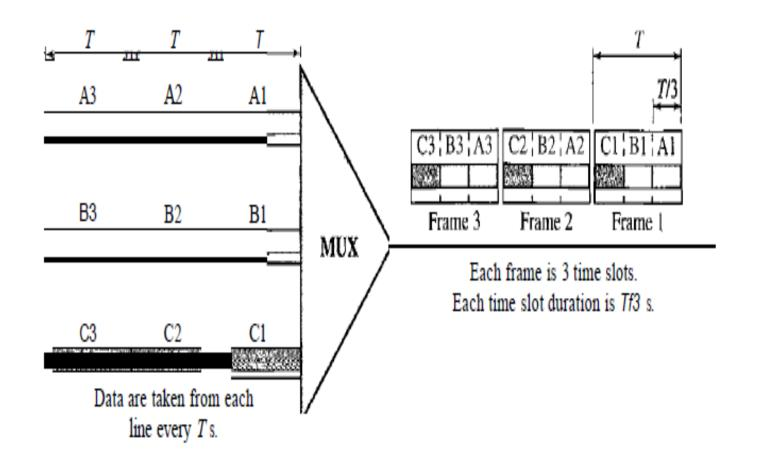
Input unit duration = T **Output unit duration** = T/n, ( n input connection) **Frame duration** = Input unit duration (T) Frame rate = Input rate **Date rate**= 1 / unit duration **Unit Duration** = 1/ date rate **Bit rate** = Output rate = Frame rate x Frame size
