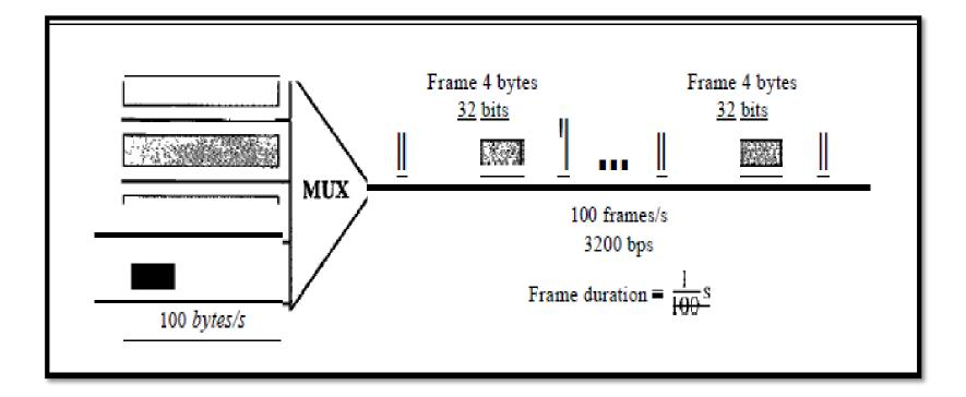
Each frame carries 1 byte from each channel; the size of each frame, therefore, is 4 bytes, or 32 bits. Because each channel is sending 100 bytes/s and a frame carries 1 byte from each channel, the frame rate must be 100 frames per second. The duration of a frame is therefore 1/100 s. The link is carrying 100 frames per second, and since each frame contains 32 bits, the bit rate is 100 x 32, or 3200 bps. This is actually 4 times the bit rate of each channel, which is  $100 \ge 8 = 800$  bps.
