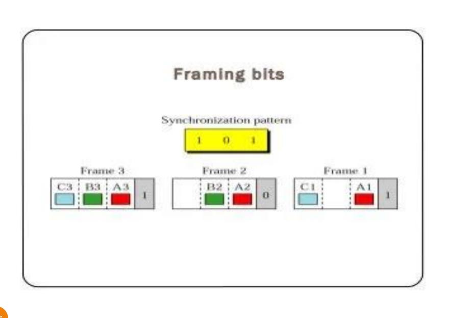
We have four sources, each creating 250 characters per second. If the interleaved unit is a character and 1 synchronizing bit is added to each frame, find (a) the data rate of each source, (b) the duration of each character in each source, (c) the frame rate, (d) the duration of each frame, (e) the number of bits in each frame, and (f) the data rate of the link.
