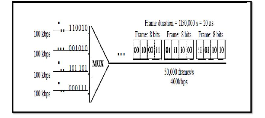
The output for four arbitrary inputs. The link carries 50,000 frames per second since each frame contains 2 bits per channel.
