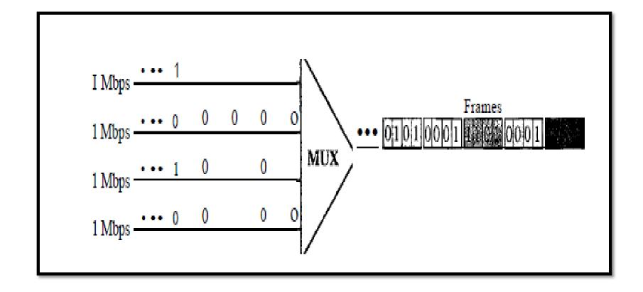
Input unit duration = 1/ input data rate =1Mbps=1/  $10^6 = 10^{-6} s = 1 \mu s$
