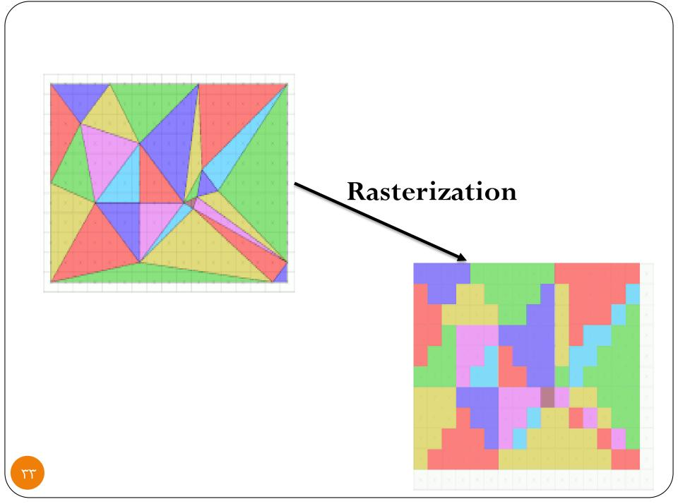
Rasterization works by taking a 3D scene made up of polygons and primitives and generating a 2D image out of it. Generally, a polygon in an application such as a video game describes a triangle made up of three points. A stream of triangles is passed to the graphics hardware, is transformed into 2D form, and is displayed to the screen. Transformations are done using various mathematical matrices.
