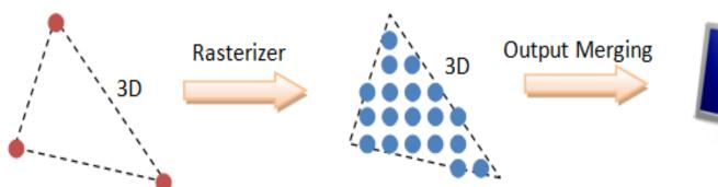
A *primitive* is formed by one or more *vertices*. Vertices are not gridaligned
